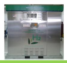
Palletized, 2 kilogram per day production, Scalable Hydrogen Fueling Appliance With 4 kilograms storage at 6,000 psi with fixed orifice fueling and J2600 nozzle J2719 fuel quality
